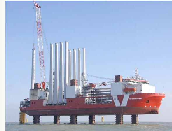
Jack Up Barge
